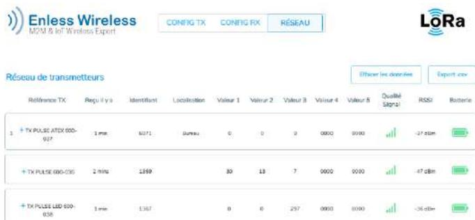
The screenshot shows the 'RÉSEAU' tab in the Enless Wireless interface. It displays a table of transmitted frames with columns for 'Référence TX', 'Requ. il y a', 'Identifiant', 'Localisation', 'Valeur 1' through 'Valeur 5', 'Qualité signal', 'RSSI', and 'Batterie'. Three frames are shown with their respective signal quality and battery levels.
